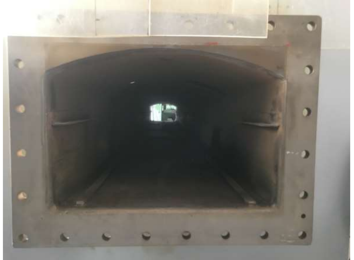
Muffle to guide gas flow close to product
