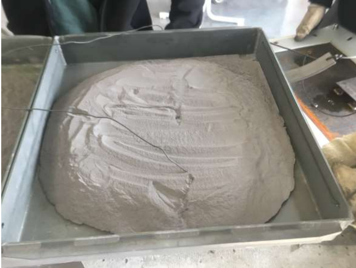
Thermocouple in powder to measure product temperature during test
